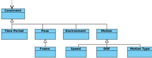
Figure 5. Constraints on skill primitives.
