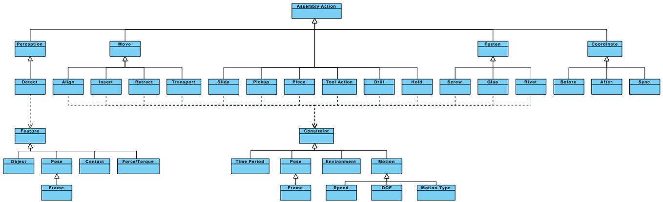
Figure 1. Taxonomy for manufacturing assembly task.
