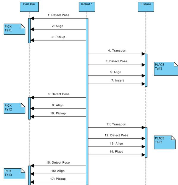
Figure 8. Sequence diagram for airplane assembly.
